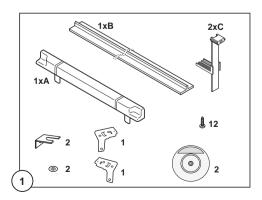
Two cabinet securing brackets are supplied with the installation pack. They need to be assembled onto the cabinet prior to cabinet being pushed into the Kitchen aperture.
